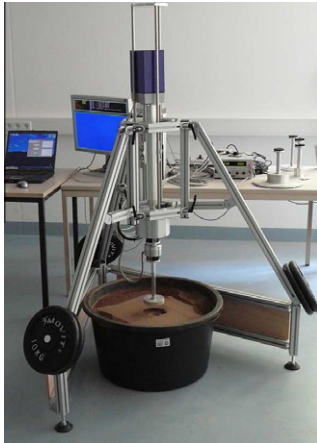
Fig. 2. Bevameter for soil characterization.
