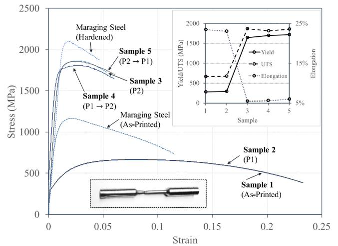
**Fig. 2.** Engineering stress-strain curves for hybrid test samples as-printed and heat-treated. Printed and heat-treated/hardened pure Maraging steel stress-strain curves are also shown as the dotted lines for comparison. The top inset summarizes the yield and ultimate stresses and elongation to failure of the five samples.
