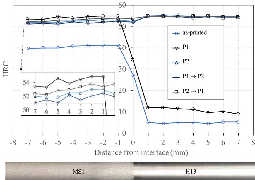
**Fig. 1.** Hardness of hybrid steel samples across the hybrid steel samples. All printed samples measured 99.8% density.
