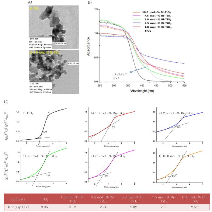
Fig. 1. TEM image (A), diffuse reflectance-UV-visible absorption spectra (B), and their Tauc's plots (C) of the prepared Bi-TiO<sub>2</sub> powders.
