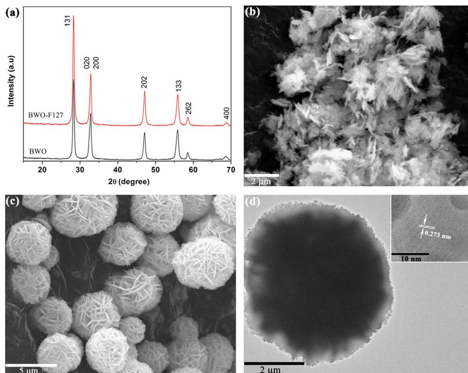
Fig. 1. (a) XRD patterns, (b) SEM image of BWO, (c) SEM image of BWO-F127, (d) TEM image of BWO-F127 (inset is the corresponding HRTEM image).
