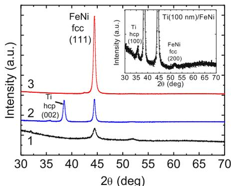
Fig. 1. X-ray diffraction spectra for FeNi(100 nm) (1), Ti (100 nm)/FeNi (100 nm) (2) and Ti (10 nm)/FeNi (100 nm) (3) films. Inset shows X-ray diffraction pattern for Ti (100 nm)/FeNi (100 nm) film at lower scale.
