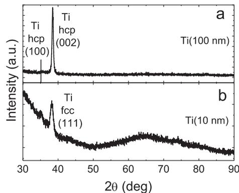
Fig. 2. X-ray diffraction spectra for Ti (100 nm) (a) and Ti (10 nm) (b) films.
