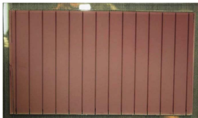
Fig. 1. Anode plate with robust current collecting fingers.
