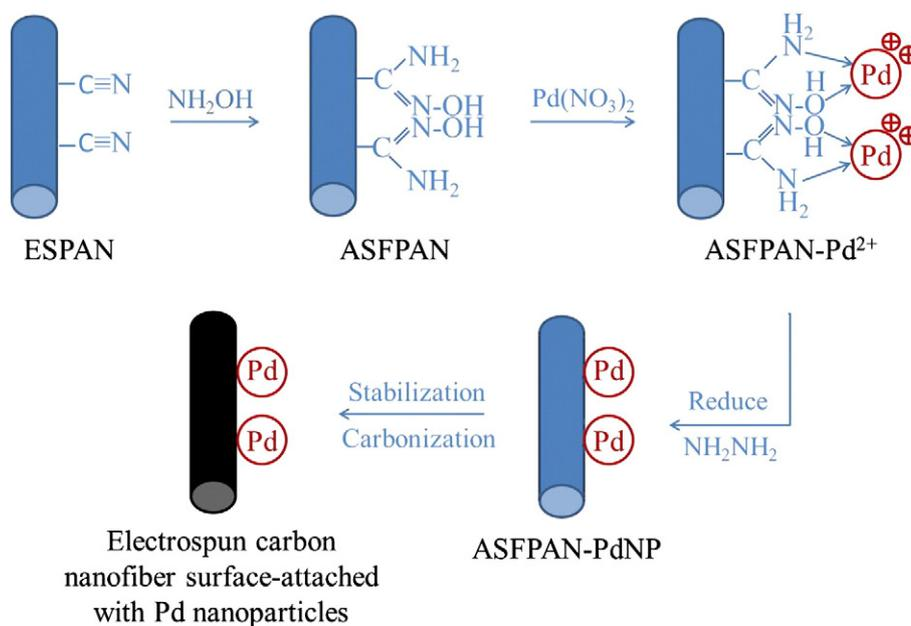
Fig. 1. A schematic representation showing all of the steps for the preparation of electrospun carbon nano-felt surface-attached with Pd nanoparticles.
