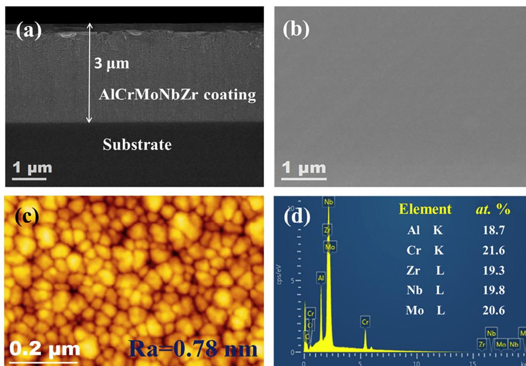
Fig. 1. (a) Cross-sectional SEM image of the coating; (b) surface morphology of the coating; (c) surface AFM image of the coating; (d) corresponding EDS spectra.
