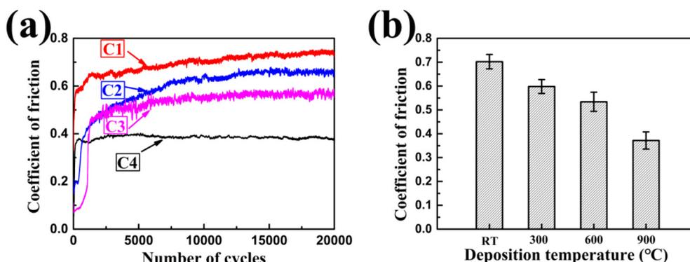
Fig. 1. Coefficient of friction curves as a function of sliding cycles (a), and average values for YSZ coatings deposited at different deposition temperatures.
