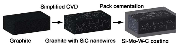
Fig. 1. Diagram of preparing SiC nanowire-toughened Si-Mo-W-C coating on the graphite.
