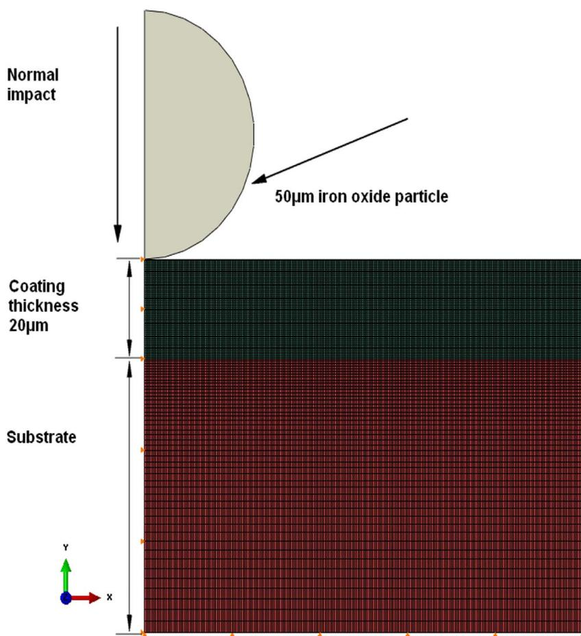
Fig. 1. Typical 2D axisymmetric FE model with fine mesh and boundary conditions used to investigate solid particle erosion of coated systems.
