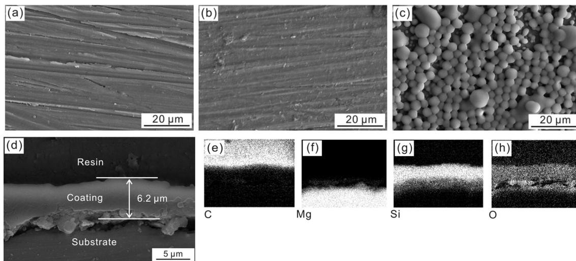
Fig. 2. SEM images of (a) AZ31 alloy, (b) (PAA/GS)<sub>20</sub>/Mg and (c) PMTMS/(PAA/GS)<sub>20</sub>/Mg, (d) cross-sectional SEM image and (e–h) element mapping of PMTMS/(PAA/GS)<sub>20</sub>/Mg.
