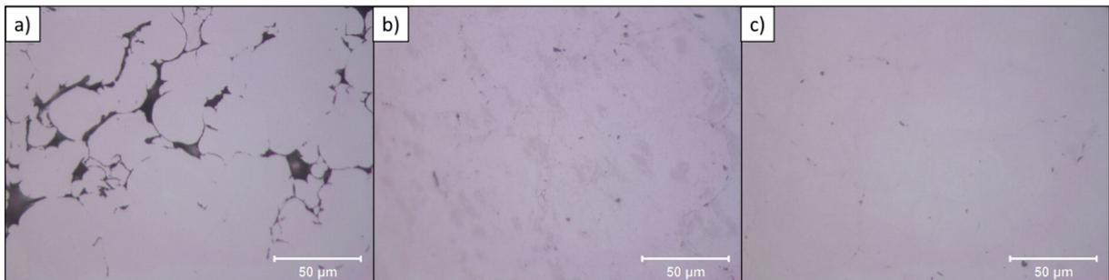
**Fig. 1.** Top view LOM images of Ti cold spray coatings: a) CS1, b) CS2 and c) CS3.
