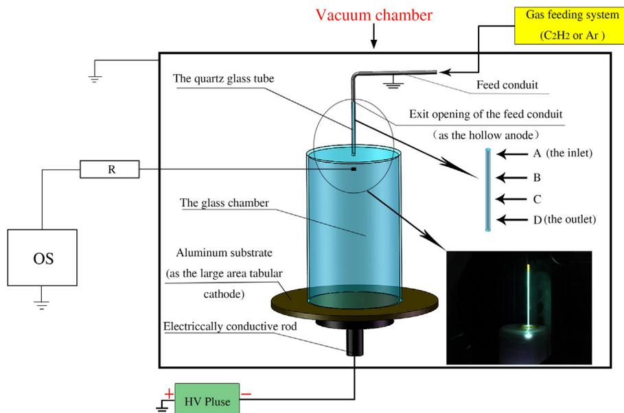
Fig. 1. Schematic of the EGD-PIII&D system for inner surface treatment of quartz tubes.
