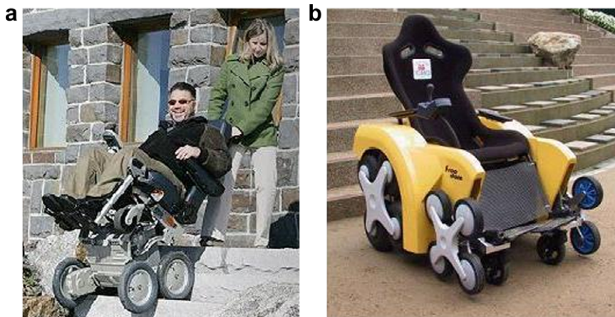
Fig. 1. Examples of existing of staircase climbing vehicles: (a) wheelchair iBOT with two-wheel clusters, [2]; (b) Tamagawa staircase climbing wheelchair Freedom with four wheel clusters, [3].
