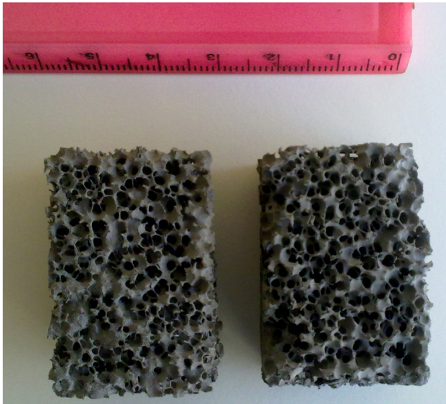
Fig. 1. Samples of the open cellular Ti6Al4V alloy based foams produced via replication and powder metallurgy techniques.
