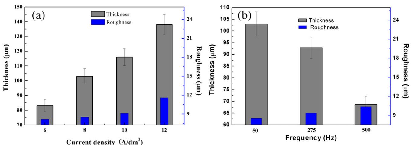
**Fig. 1.** Thickness and roughness of the coating prepared under different current densities and working frequencies.
