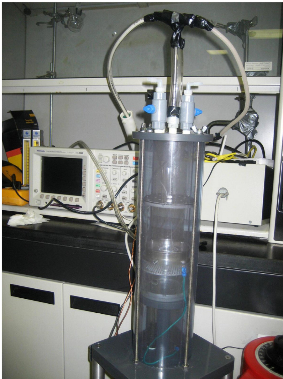
Fig. 1. A photo and cross-sectional schematic diagram of the corona discharge plasma reactor.
