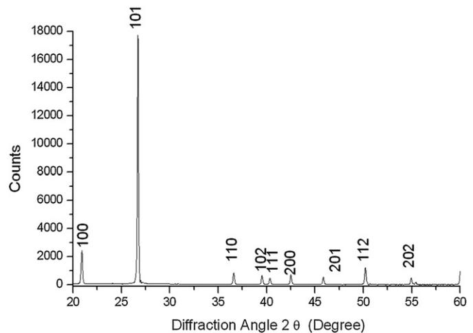
Fig. 2. XRD pattern of SiO<sub>2</sub> powder.
