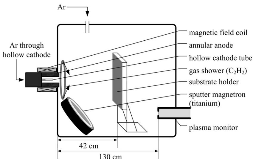
Fig. 1. Side view on the vacuum chamber. The arrows at the gas shower indicate the acetylene flow direction into the external plasma.
