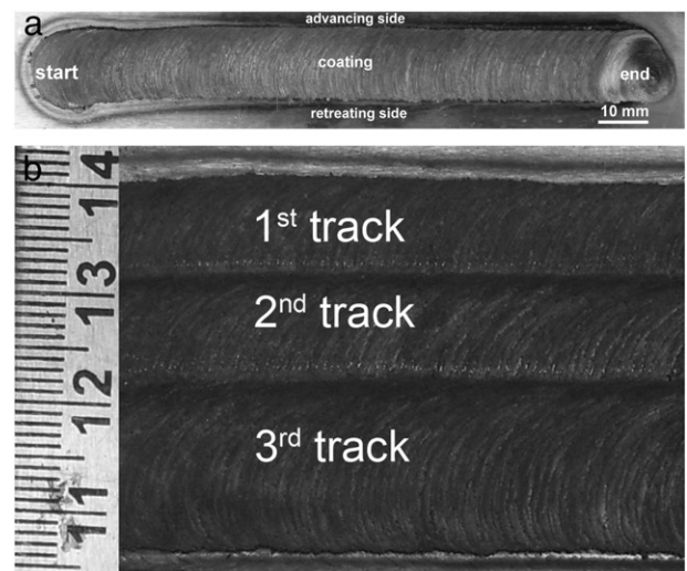
Fig. 2. Typical single-track (a) and multi-track (b) friction surfaced coatings in alloy 440C.
