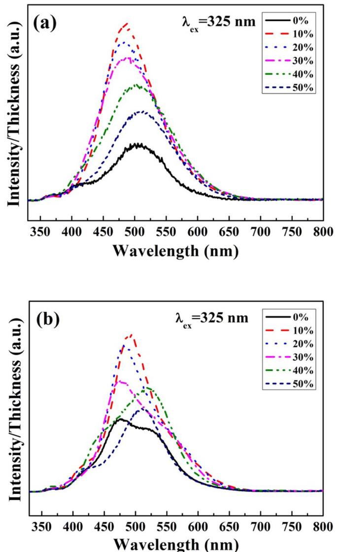
Fig. 2. Room temperature PL spectra of the Bi-doped Y<sub>2</sub>O<sub>3</sub> thin films with (a) a 300 nm thickness level and (b) a 500 nm thickness level as a function of O<sub>2</sub> content in the sputtering atmosphere.
