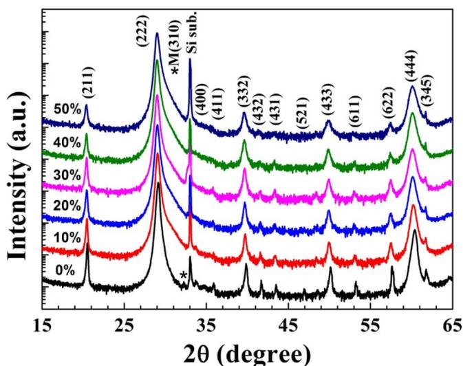
Fig. 1. XRD patterns of the Bi-doped Y<sub>2</sub>O<sub>3</sub> thin films with a 300 nm thickness level depending on oxygen content in the sputtering atmosphere.
