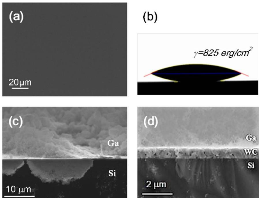
Fig. 1. (a) FE-SEM image of the WC/Si(111) surface, and (b) contact angle measurements of the surface energy. Cross-section images of (c) Ga/Si(111) and (d) Ga/WC/Si(111) samples. Evidence of a Ga-Si reaction was observed from Fig. 1(c).
