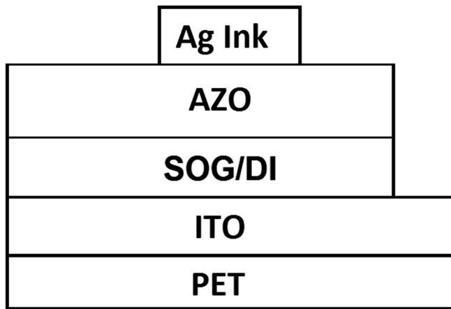
Fig. 1. Schematic structure of the flexible MIS diodes.
