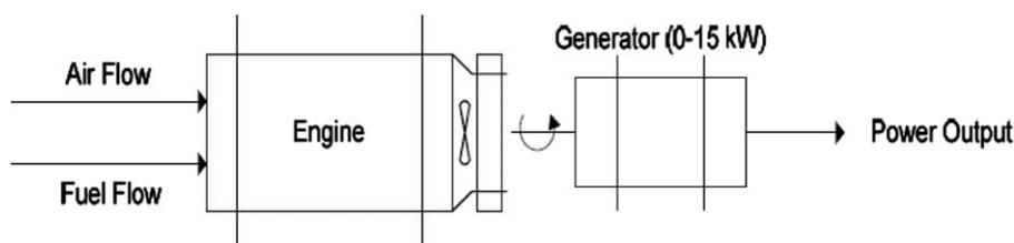
**Fig. 1.** Schematic of the engine/generator set.
