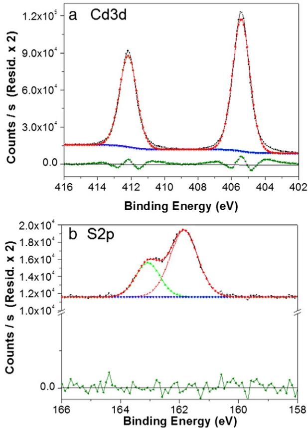
**Fig. 1.** The XPS spectra measured for pulsed DC deposited CdS, was not affected by the deposition conditions, showing photoelectron core levels of (a) Cd3d<sub>5/2</sub> and Cd3d<sub>3/2</sub> and (b) S2p for CdS thin films deposited at 10 sccm Ar, 500 W and 150 kHz. For (a) the fitting is achieved with a single Gaussian peak due to CdS and for (b) the fitting shows the splitting of S2p<sub>3/2</sub> and S2p<sub>1/2</sub>. The green line below shows the error fitting function.
