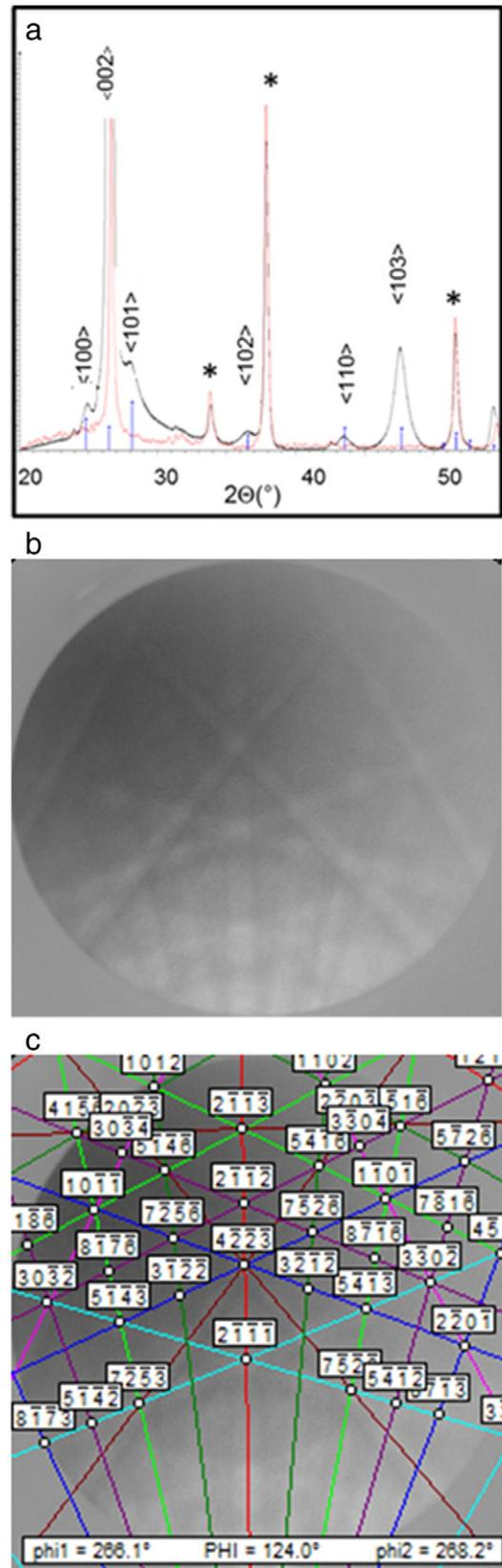
**Fig. 2.** (a) XRD pattern, (b) Kikuchi pattern and (c) Kikuchi phase map of a CdS film sputtered on TEC15 coated glass for 3600 s, 10 sccm Ar, 500 W, 150 kHz, 2 s (ramp time), 2 μs (reverse time). The \* in (a) indicates peaks due to the TEC 15 glass substrate.
