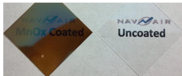
Fig. 1. PECVD synthesized \text{MnO}_x film (on left) coated on a glass cover slip and an uncoated glass cover slip (right).
