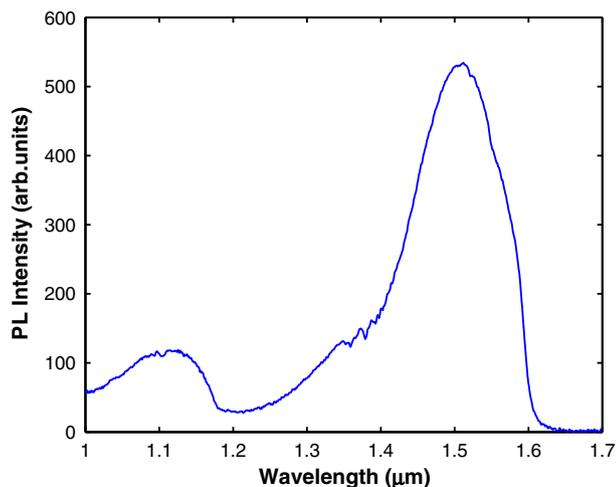
Fig. 2. Room-temperature PL spectrum of the sample with three layers of Ge QDs grown on SOI.
