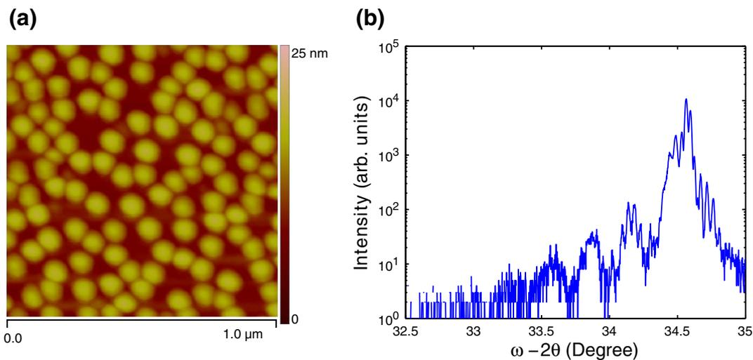
Fig. 1. (a) AFM image of the first layer of Ge QDs grown on SOI. (b) XRD rocking curve of the sample with three layers of Ge QDs grown on SOI.
