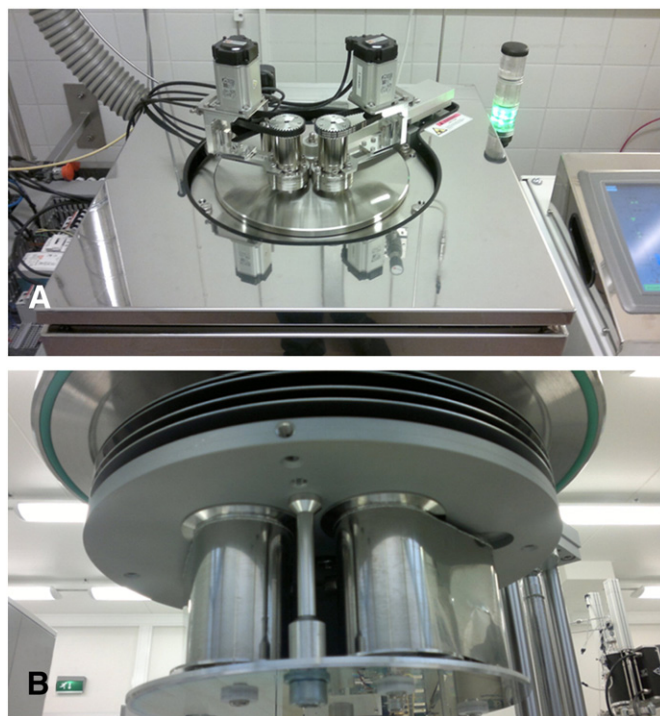
Fig. 1. R2R setup assembled to a batch ALD reactor (A) and the R2R mechanism (B).
