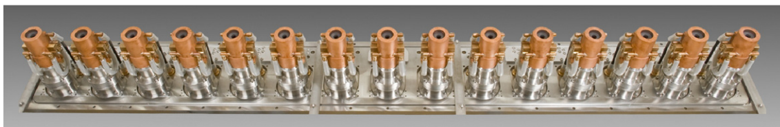
Fig. 3. Arrangement of a number of hollow cathode arc (hca) sources to apply plasma enhancement over a width of 2.85 m; hca-sources are mounted on a rectangular flange right to be installed in web coating machines.
