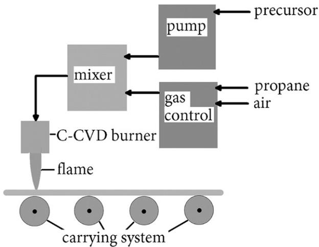
Fig. 1. Sketch of the coating system used.
