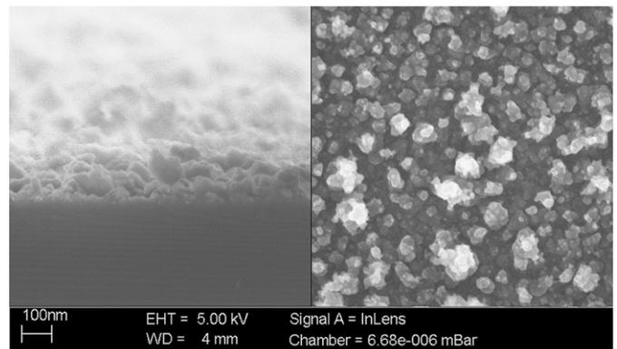
Fig. 2. Typical morphology of the ZnO thin films coated by C-CVD at atmospheric pressure as observed by SEM. Left: cross section, right: top view.
