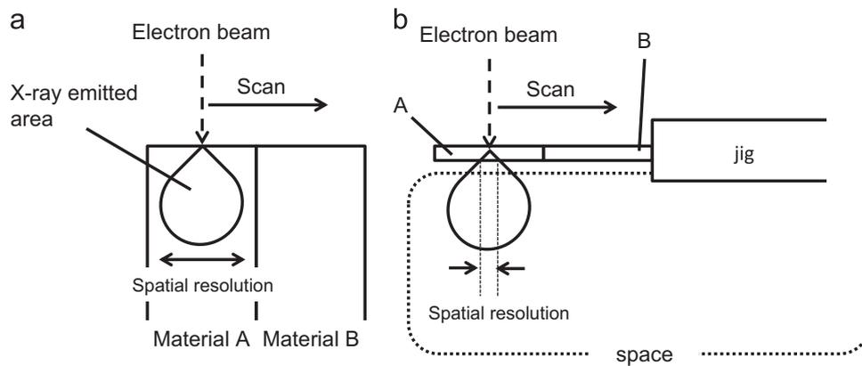
**Scheme 1.** Concept of spatial resolution improvement in FE-EPMA by sample thinning. (a) Bulk-sample FE-EPMA and (b) thin-sample FE-EPMA. From (a) and (b), it is evident that sample thinning improves the spatial resolution and the detection sensitivity is worsened due to the reduction in sample volume.
