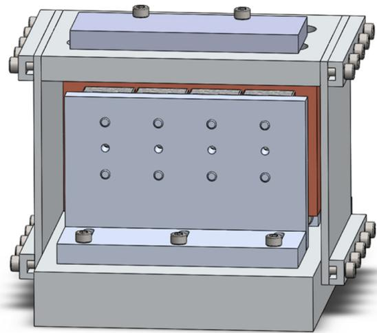
**Fig. 3.** Flexure with embedded eddy current damper.
