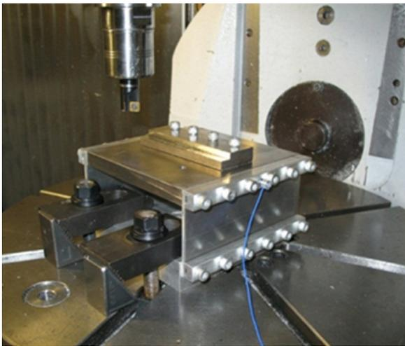
**Fig. 1.** Example parallelogram, leaf-type flexure used for milling experiments. A workpiece is mounted to the top of the flexure, an accelerometer is used to measure the vibration during cutting, and an inserted cutting tool is pictured.
