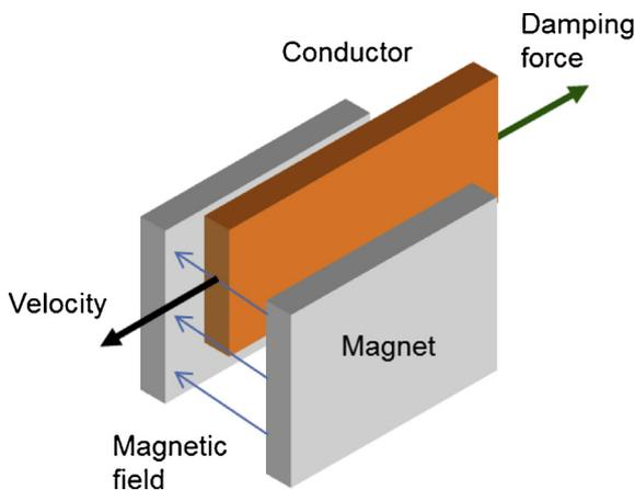
**Fig. 2.** Schematic of an eddy current damper.
