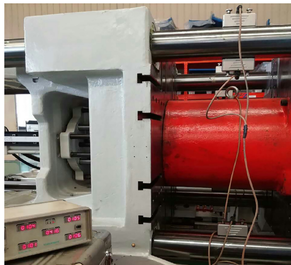
(c) Picture of spot installation of measuring device
