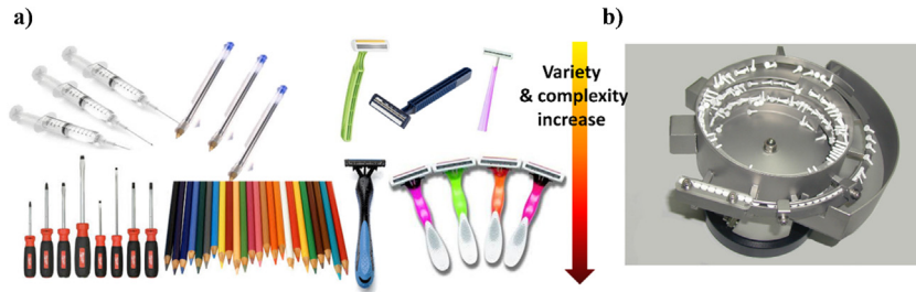
Fig. 1. (a) Variety of products in consumer goods industry and (b) feeder bowls.
