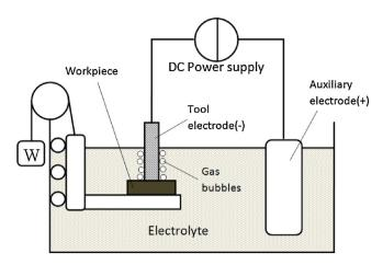
Fig. 1. Schematic view of ECDM setup using gravity feeding system.
