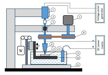
**Fig. 2.** Schematic view of vibration assisted ECDM setup: (1) piezoelectric actuator, (2) polymeric insulating part, (3) coupling bearing, (4) tool holder (chuck), (5) tool electrode, (6) workpiece, (7) electrical DC motor, (8) belt and pulley system, (9) counter electrode (anode), (10) workpiece holder connected to the linear guide way, (11) x–v table.
