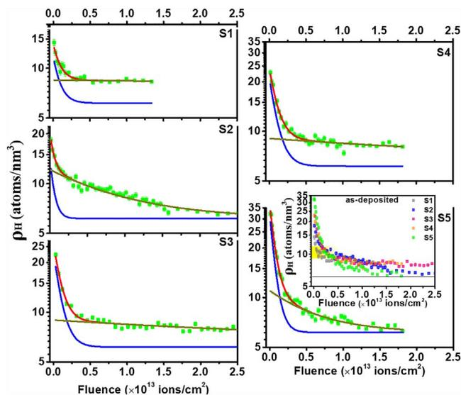
Fig. 1. Hydrogen concentration profiles as measured in the ERDA experiment for as-deposited  $\alpha$ -SiN<sub>x</sub>:H thin films S1 to S5 and their fitting with two exponentials decays, which represent different hydrogen release mechanisms. Inset shows the data overlapped on one another, wherein the yellow strip indicates the H concentration below which the H release slows down significantly.
