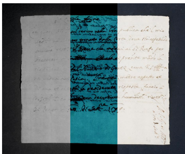
Fig. 1. Manuscript photographed in NIR (950 nm), UV and VIS respectively. Recorded ink migrations and document preservation state are comparatively shown. The UV photograph shows a thick halo of absorbed UV radiation around the original pen stroke (best seen in the NIR photograph) indicating the spread of ink component migrations. Strong radiation absorption, as well as some fluorescence in the location of the text verso, is also seen. No further stains, burn-troughs or cracks have been revealed under UV or NIR that has not already been detected under day light.
