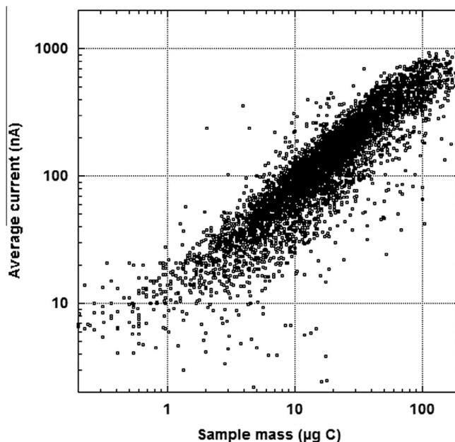
Fig. 1. Measured current of 12 MeV  $^{13}\text{C}^{3+}$  ions after the high energy magnet in nA as a function of the mass of the samples in  $\mu\text{g}$  of carbon for 6672 samples. The plot is shown on a log–log scale.
