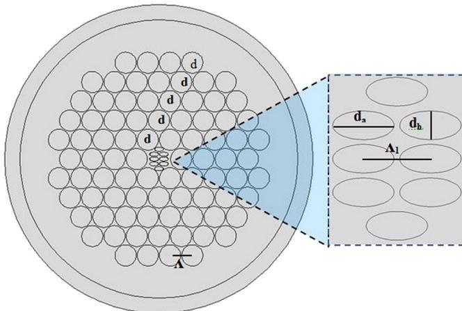
Fig. 1. Transverse cross section of the proposed E-PCF.
