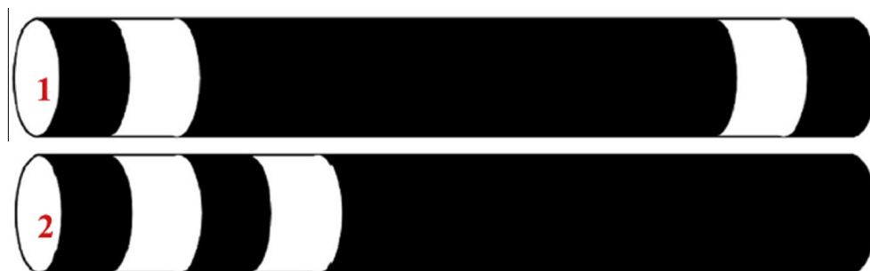
Fig. 1. Schematic plot of the two different electrode configurations. The black stripes show the single electrodes along the outer surface of the glass capillary.
