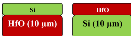
Fig. 1. Schematic image of the light-on-heavy (left) and heavy-on-light (right) configurations that were used in our simulations. The thickness of the top layer was varied and the thickness of the substrate layer was chosen to be much larger than the interaction volume of the helium beam.
