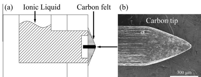
Fig. 2. Developed ionic liquid ion source: (a) schematic diagram of ionic liquid ion source and (b) SEM image of emitter tip made of graphite rod.
