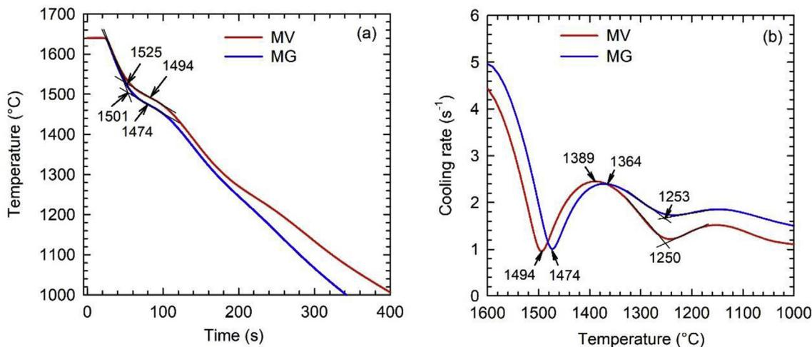
**Fig. 1.** Experimentally measured cooling curves for MV and MG sample: (a) Dependence of temperature on time; (b) Dependence of cooling rate on temperature. The phase transformation temperatures are indicated in the figures.
