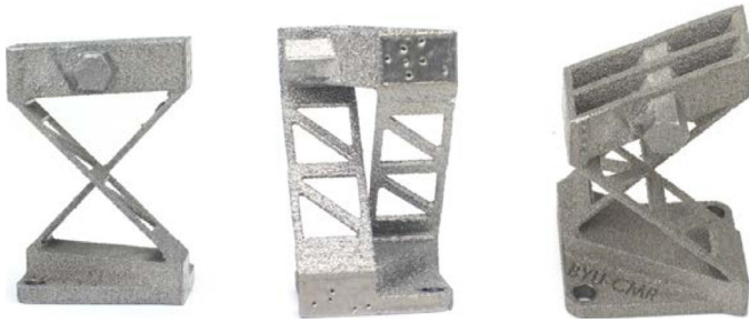
Fig. 1. A 3D printed titanium cross-axis flexural pivot with an early lattice flexure design.
