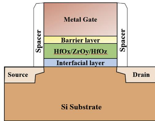
Fig. 2. Schematic profile of a HK/MG MOSFET.
