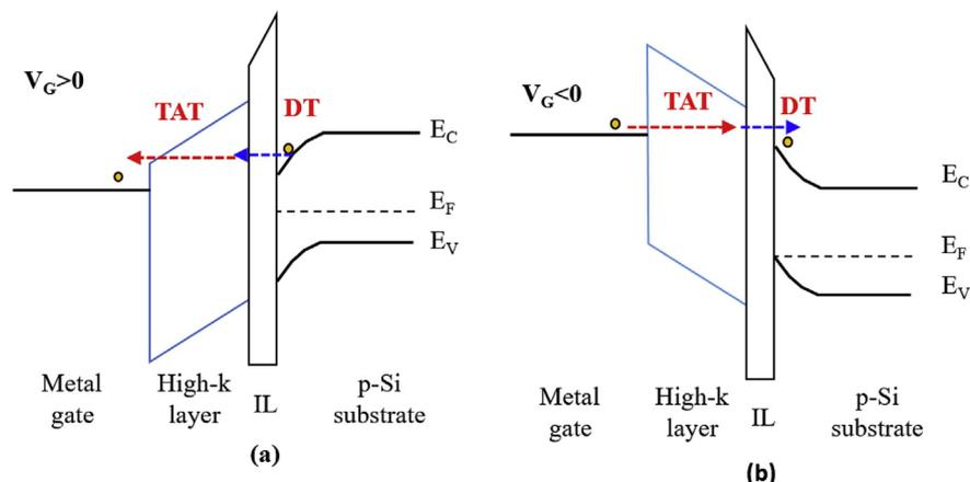
Fig. 1. Band diagram with trap assisted tunneling through high-k layer and interfacial layer of (a) positive gate bias and (b) negative gate bias.
