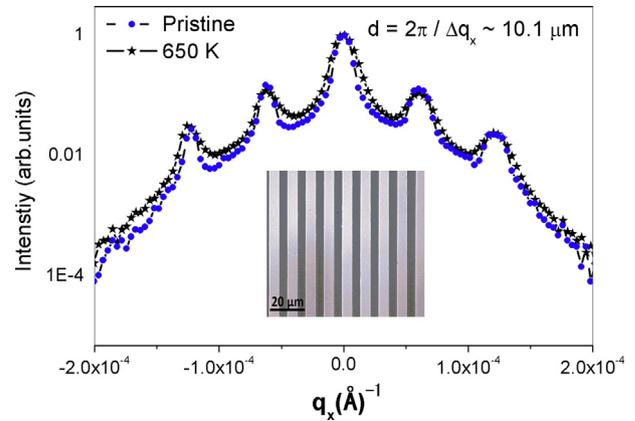
Fig. 1. X-ray rocking curve scans of pristine and 650 K annealed patterned Fe/Pt multilayer. Incident x-rays are perpendicular to the length of pattern stripes. From the separation of peaks ( $\Delta q_x$ ) grating periodicity ( $d$ ) is calculated. Inset shows the optical image of the patterned Fe/Pt multilayer after lift-off process.
