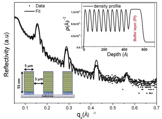
Fig. 2. X-ray reflectivity (XRR) data of pristine patterned Fe/Pt multilayer sample. Symbols are the experimental points and the solid line is the best fit to the data. Bottom inset shows the schematic of patterned Fe/Pt multilayer and the top inset shows the electron density profile along the depth of multilayer as obtained from the fitting of XRR pattern.
