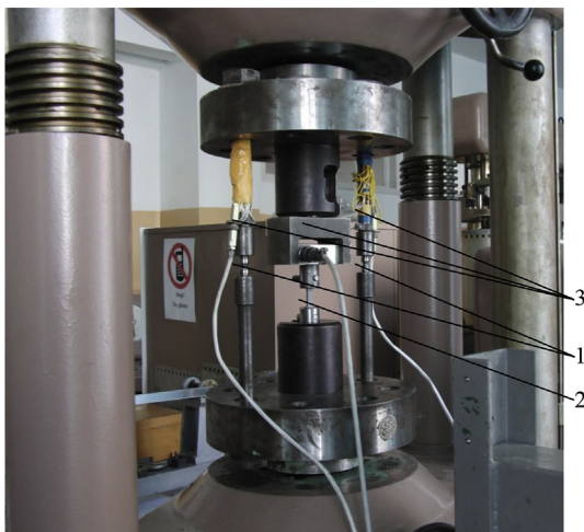
Fig. 1. General view of appliance for realization of impact-oscillatory loading; 1–“brittle” specimens; 2–central specimen; 3–dynamometers.
