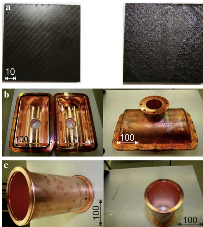
Fig. 1. a. CFRP sample before coating (front and backside), b. Cu coated CFRP vacuum chamber, c. Cu coated CFRP vacuum tube. Three different test pieces were used to investigate the vacuum properties of copper-coated CFRP. The square CFRP sample (a) was first characterized without coating, later with. A custom made model (b) of a possible later application was made using one aluminum negative to make two half shells. A standard, “off-the-shelf”, CFRP tube (c) was fitted with two custom made ISO-K DN160 flanges to demonstrate that the technology can be used to produce standard vacuum parts (all scales inserted in the pictures are in mm).
