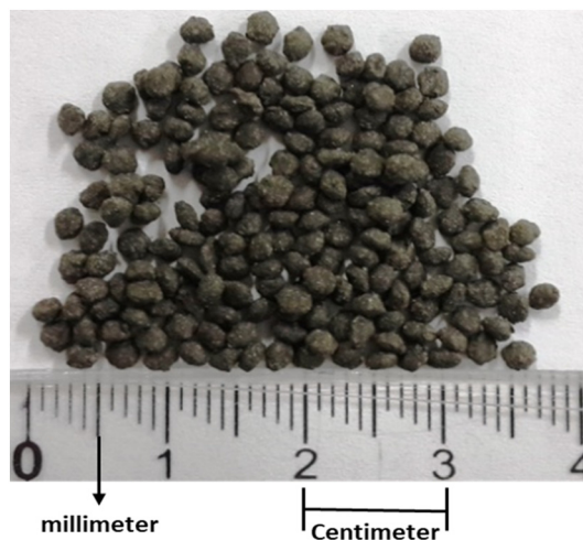
Fig. 1. Photograph of iron oxide modified clay-activated carbon composite beads.
